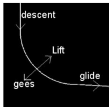
My design with its larger wings (lower **wing loading**) was to perform this pull-up manoeuvre at a higher altitude than Burt's, which would lessen the gees and extend the glide distance, especially as my design remained supersonic at the end of the pull-up unlike SS2.
