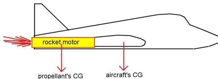
However, as propellant is jettisoned out the nozzle, the remaining propellant mass decreases, and unfortunately, the propellant's own C.G. is significantly rearwards of the overall aircraft C.G. So the tail gets progressively lighter, making the aircraft progressively nose-heavy (the overall C.G. moves nosewards), which requires more and more elevator deflection to keep in trim and prevent a nosedive. The required elevators can get excessively large and draggy.
