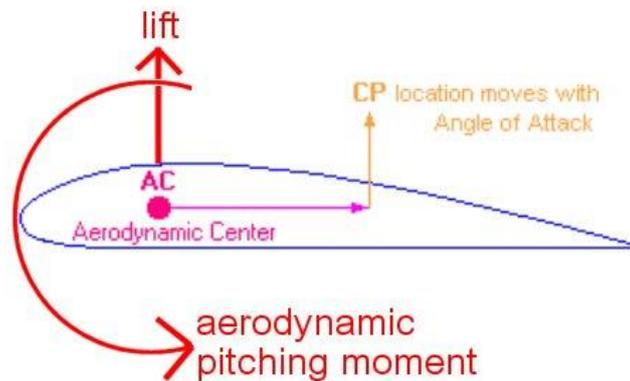
This is done because when you analyse traditional aircraft wings, you can find a position for the lift vector, (labelled the *Aerodynamic Centre A.C.*) where this A.C. doesn't move with angle of attack up to the wing stall. This is preferred to the centre of pressure because the center of pressure moves fore and aft with changing wing angle of attack.
