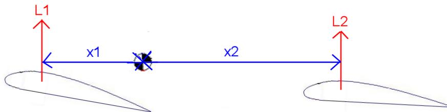
The forward wing is bolted-on at double the angle of attack of the rear, so is lifting with double the force of the rear. Therefore the C.G. (pivot of the see-saw) has to be nearer the front wing to keep balance: distance  $x_1$  is half of distance  $x_2$ .
