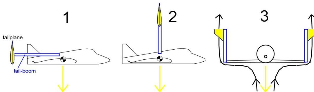
But this would mean that the tailplane would be in the dead air of the wake; it wouldn't work. At this point I gave up, but Burt didn't. He realised that he could modify the tailboom of picture 2 by splitting it in two and bolting it to the wingtips. As the front view of picture 3 shows, the tailfins are now in the moving air flowing past the vehicle so will function properly. And that's why Burt is a genius!
