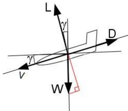
Or to put it another way, if your lift-to-drag ratio is four, you'll glide 4 metres forward for every metre of height lost, in still air. This lets you calculate the aircraft's lift-to-drag ratio if you can measure its glide angle (measure its height loss and distance travelled forward).
