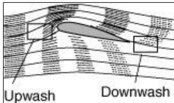
This upwash affects the canard angle of attack, and the downwash affects the tailplane angle of attack, we need to be able to account for these washes.
