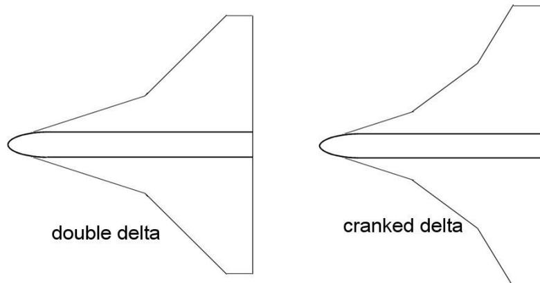
The powerful vortices forward energise the less powerful vortices rearward to literally keep them spun-up at high angles of attack. Therefore, double-delta wings and their modern equivalent: cranked delta wings, can fly at much higher angles of attack which reduces their landing airspeed.
