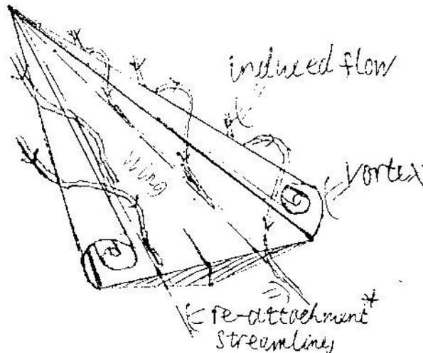
This spinning tame whirlwind induces flow above the vortex, which would otherwise be stalled at such a high angle of attack, to flow back down onto the wing.
