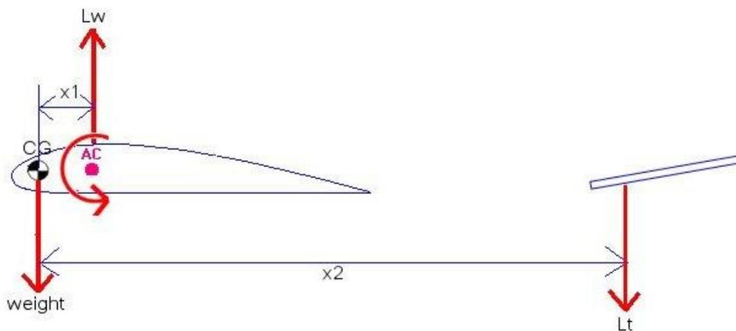
Note that this equation works just as well for canard aircraft, where the lift of the canard  $L_C$  is now upward (positive):
