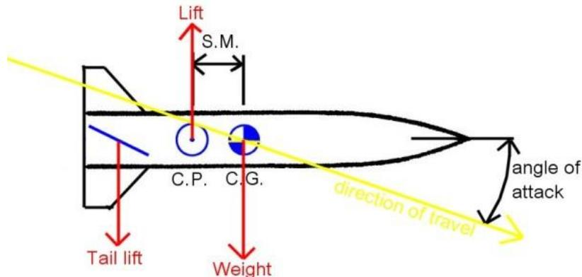
Now the vehicle is gliding: the direction of travel (of the C.G.) is shown here in yellow. The C.P. and C.G. are not coincident (finite Static Margin for stability) but this unfortunately creates a nose-down pitching moment (called a 'couple') in the pitch axis: the lift and the weight are pulling in opposite directions, but are some distance apart.
