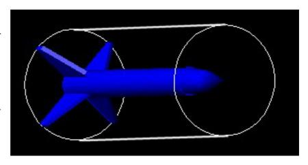
When the air flows through the gap between each fin, the cross-sectional area available to the air between the fuselage and the edge of our tube is reduced by the bulk of the fins. At subsonic speeds, the air simply speeds up temporarily as it flows through this restriction in accordance with Bernoulli's principle.
