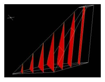
A mathematical upshot of the area rule is that if it isn't possible to keep the cross sectional area constant right down the fuselage, then any changes in area must occur as slowly as possible with distance down the fuselage (rate of change of area with fuselage distance.) Consequently, it's important to bevel the trailing edges of straight deltawing fins otherwise there's a sudden decrease in cross-sectional area at the trailing edge.
